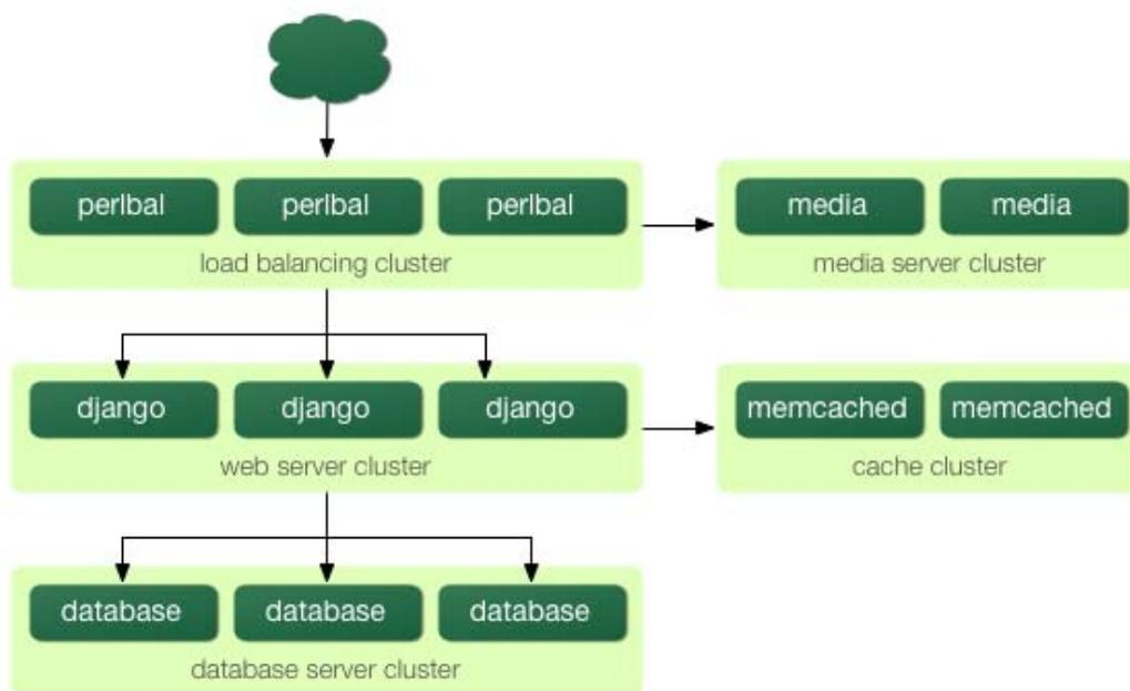
2 Though we’ve only shown two or three servers at each level, there’s fundamentally no limit to how many you can add.
