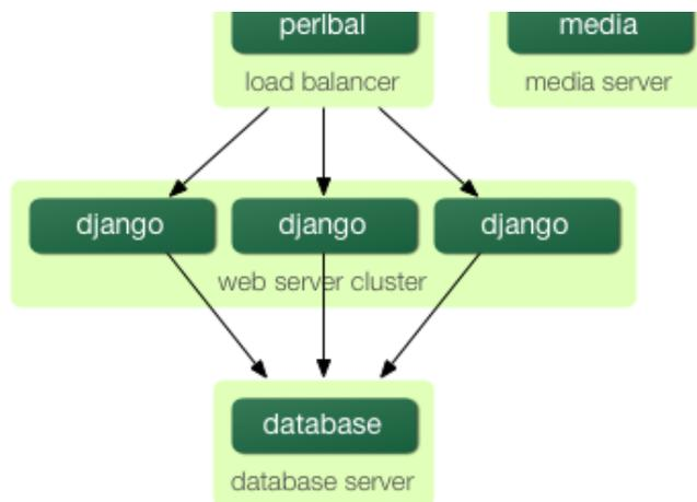
Notice that in the diagram the web servers are referred to as a “cluster” to indicate that the number of servers is basically variable; once you have a load balancer out front, you can easily add and remove backend web servers without a bit of downtime.
