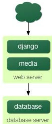
Here we're starting to move into what's usually called **N-tier** architecture. Don't be scared by the buzzword: it just refers to the fact that different "tiers" of the web stack get separated out onto different physical machines.
